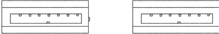
Figure 3: Using SeriTek/2ME4-E with a drive enclosure that has I-shaped eSATA connectors; both cable connectors will be identical.
